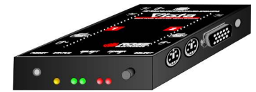
Model KVT-2PC 2-port PC connectors with audio
